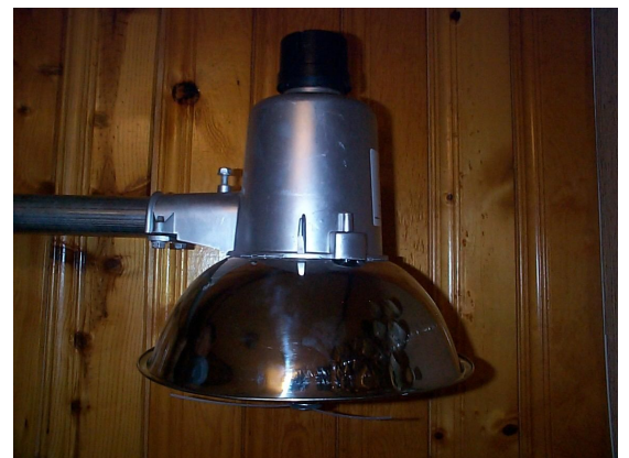
Once the bugs come to the light, an electric motor with weed-eater type blade, knocks the bugs into the water. --- Dinner is served!
